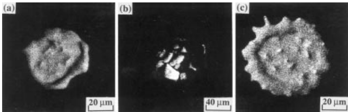
Fig. 5 Typical \text{N } K_\alpha images of EPMA of (a) titanium, (b) aluminum, and (c) TiAl compound splat (particle size: 32 to 38 \mu\text{m} , added \text{N}_2 : 17 \times 10^{-6} \text{ m}^3/\text{s} ).
